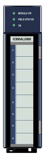
Universal Analog Input module IC695ALG600 provides eight general purpose input channels and two Cold Junction Compensation (CJC) channels. Inputs are divided into two equal groups of four. Channels can be individually-configured using the Machine Edition software for:
